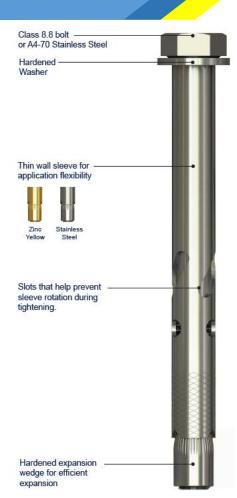
Hobson Tygabolts® are pre-assembled single unit wedge type anchors that are used in solid concrete applications. Fixing is achieved by controlled torqueing of the nut which draws the cone section up into the sleeve, thereby expanding it outward and forcing the Tygabolt™ against the sidewall of the pre-drilled hole.
