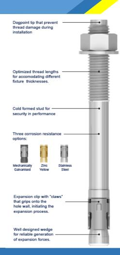
CLAWBOLTS® (Through Bolts) are preassembled single unit wedge type anchors used in solid concrete applications. Fixing is achieved by controlled torqueing of the nut which draws the tapered section up into the clip, thereby expanding it outward and forcing the CLAWBOLT® against the sidewall of the pre-drilled hole.
